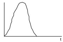
Since F is not constant the impulse (Ft) is equal to the **area** under the graph. In any calculation involving impulse the unbalanced force calculated is always the average force and the maximum force experienced would be greater than the calculated average value.
